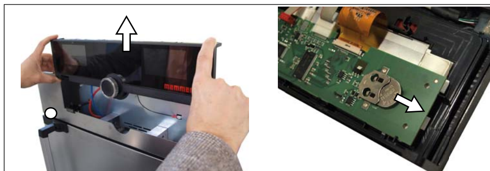
Fig. 26 Removing the lithium battery
